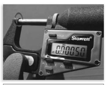
A Starrett micrometer is used to measure a sheet of stainless steel, which, at 0.0005 inch thick, is thinner than paper. Brewster Washers uses the sheet to make a thin washer to precisely level missile guidance systems. The washer is in the upper left corner of the photo. Photo courtesy of Brewster Washers.
